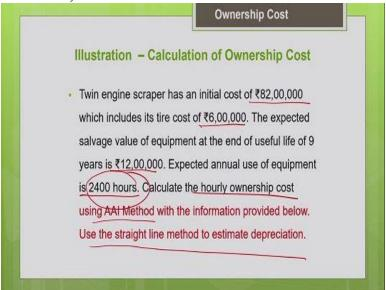
Now, let us work out an example on how to estimate the ownership cost of the machine using average annual investment method a twin engine scraper machine as an initial cost of 82 lakhs. So, this includes its tire cost of 6 lakh, the expected salvage value of the equipment at the end of the useful life of 9 years is 12 lakh. So, the useful life of the machine is 9 years, at the end of the 9 years I will be able to sell the machine at a price of 12 lakh.
